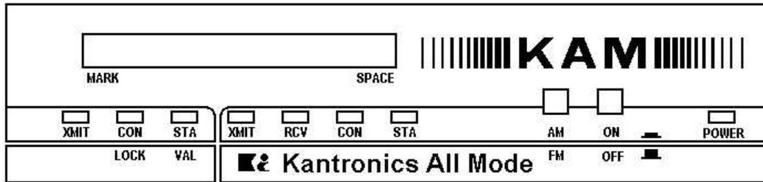
The front panel has two switches, eight LEDs and a ten segment LED bargraph. There are seven LEDs used as operating status indicators. The front panel is divided into two sections. The left three LEDs are the indicators associated with HF operation, and the four right LEDs are the indicators associated with VHF operation. The two segments are divided by a white color bar. Each LED has the functions indicated below:
