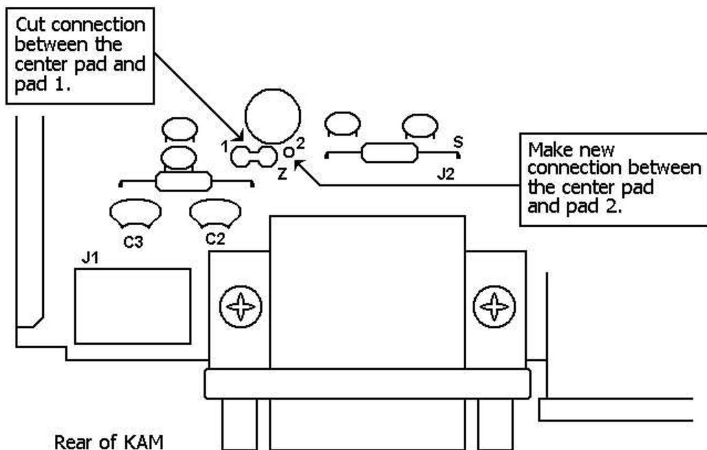
3. Locate the three pads associated with Z. Note that the center pad and the pad marked 1 is larger than the pad marked 2.
