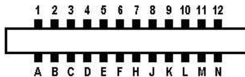
Looking at Back of computer or Back (wiring side) of connector
