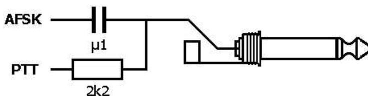
Most KENWOOD HT radios key the PTT line by connecting the sleeve of the mic connector to the sleeve of the earpiece connector. This means, that you will not need a resistor in the PTT wire from the TNC, simply connect the PTT wire to the sleeve of the mic connector. Another point to watch – most of the KENWOOD HTs (2500 and later) use a three pin mic connector. The AFSK from the TNC should therefore connect to the RING and not the TIP of the mic connector.
