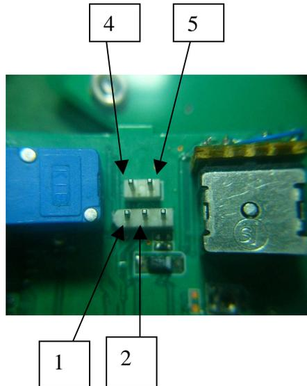
4. By using mini jumper put into terminal 1&2 and then turn on the unit, and take out mini jumper.
