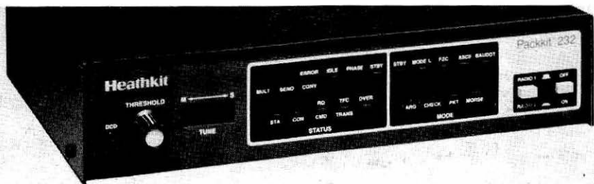
Figure 4.15—Heath HK-232 is an all-digital-mode kit that is capable of Morse, Baudot, ASCII, AMTOR and packet-radio operation. Weather facsimile picture reception is also provided.
