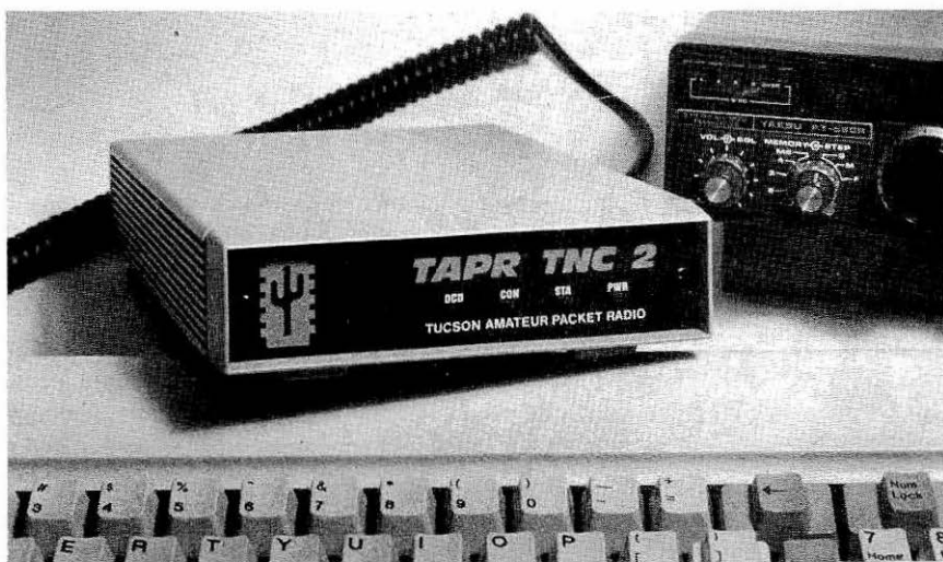
Figure 2.5—TAPR's TNC 2, the most popular TNC in amateur packet-radio history, used CMOS technology to reduce power consumption. The TNC 2 provided an advanced implementation of the AX.25 protocol.
