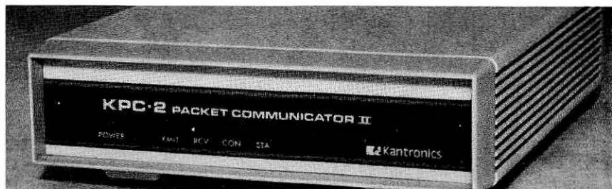
Figure 4.8—Kantronics KPC-2 TNC, a preassembled TAPR TNC-2 compatible with internal HF and VHF modems.
