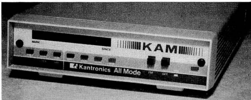
Figure 4.16—Kantronics All Mode (KAM), an all-digital-mode controller, provides gateway operation between its HF and VHF ports.
