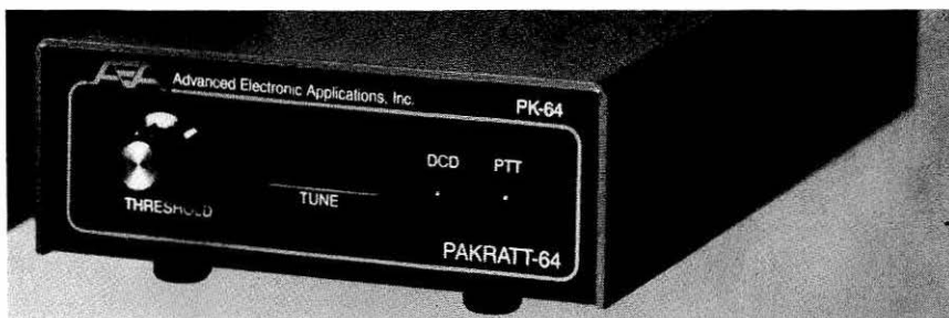
Figure 4.12—AEA PK-64 provides all-digital-mode capability for the Commodore C-64 and C-128 computers.
