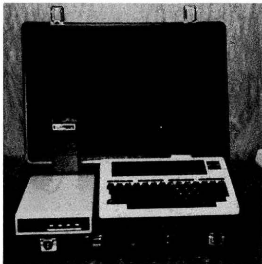
Figure 13.1—This portable packet-radio station, consisting of a TAPR TNC 2, a Radio Shack TRS-80 Model 100 laptop computer and a Tempo S1 2-meter handheld transceiver, is a versatile public-service communications tool. It can be operated at the site of an emergency or disaster and can be powered by either ac or dc.
