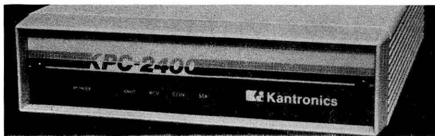
Figure 4.18—Kantronics KPC-2400 TNC, the first TNC with a modem operating above 1200 bit/s.
