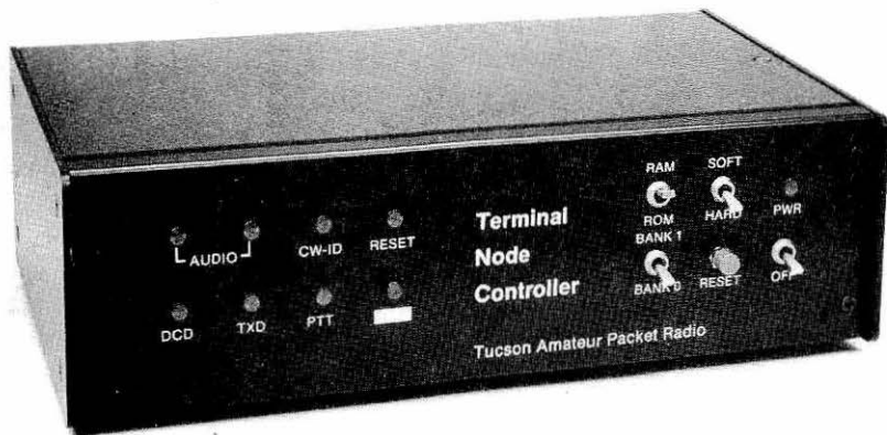
Figure 2.4 —TAPR’s TNC 1 was the first TNC to provide AX.25 protocol capability, as well as the VADCG V-1 protocol.
