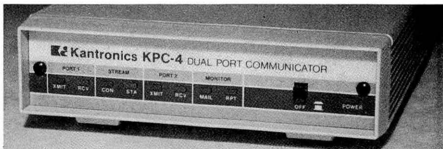
Figure 4.9—The Kantronics KPC-4 TNC permits digipeating and gateway operation between its two VHF ports. In addition, the KPC-4 includes a mailbox function.
