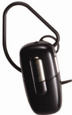
A) earset-microphone with power ON switch
